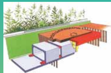
Site Preservation by Roof and Culvert Method (©Hokkaido Branch Office, East Nippon Expressway Company Ltd.)
